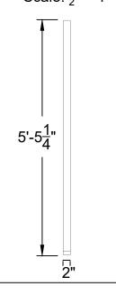
$\frac{1}{2}$ " wide  $\frac{1}{8}$ " flat sheet steel added on joints of piece J to D and K to C
